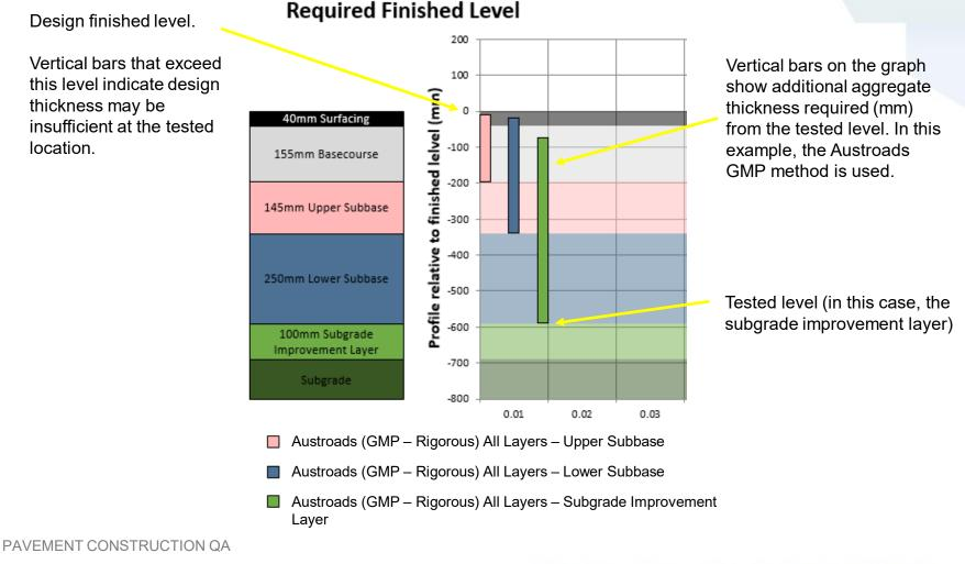
Additional aggregate thickness requirements from testing on subgrade improvement layer, lower subbase and upper subbase. Three design criteria were used here.
